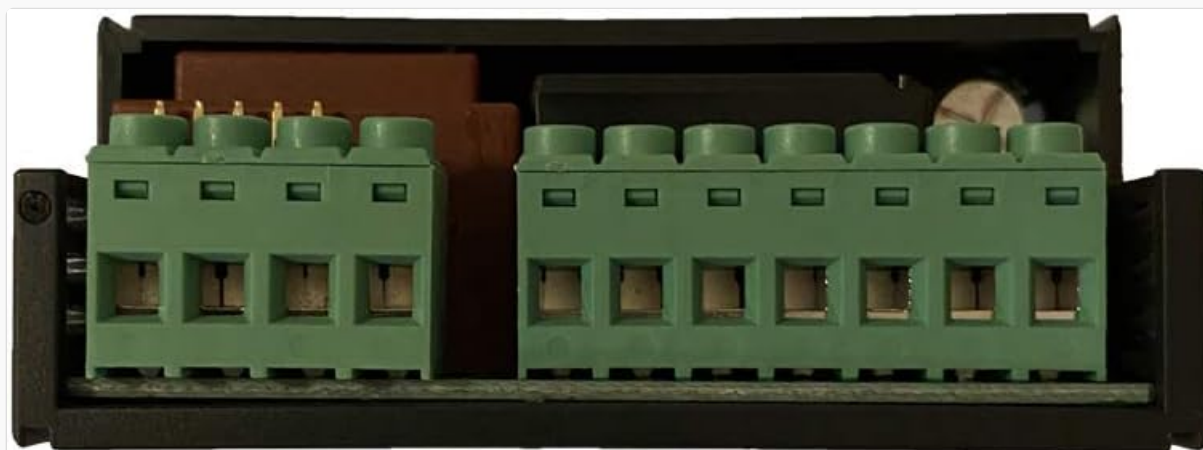
Image 4.2: Bottom view of the thermostat, highlighting the green terminal blocks for wiring.
