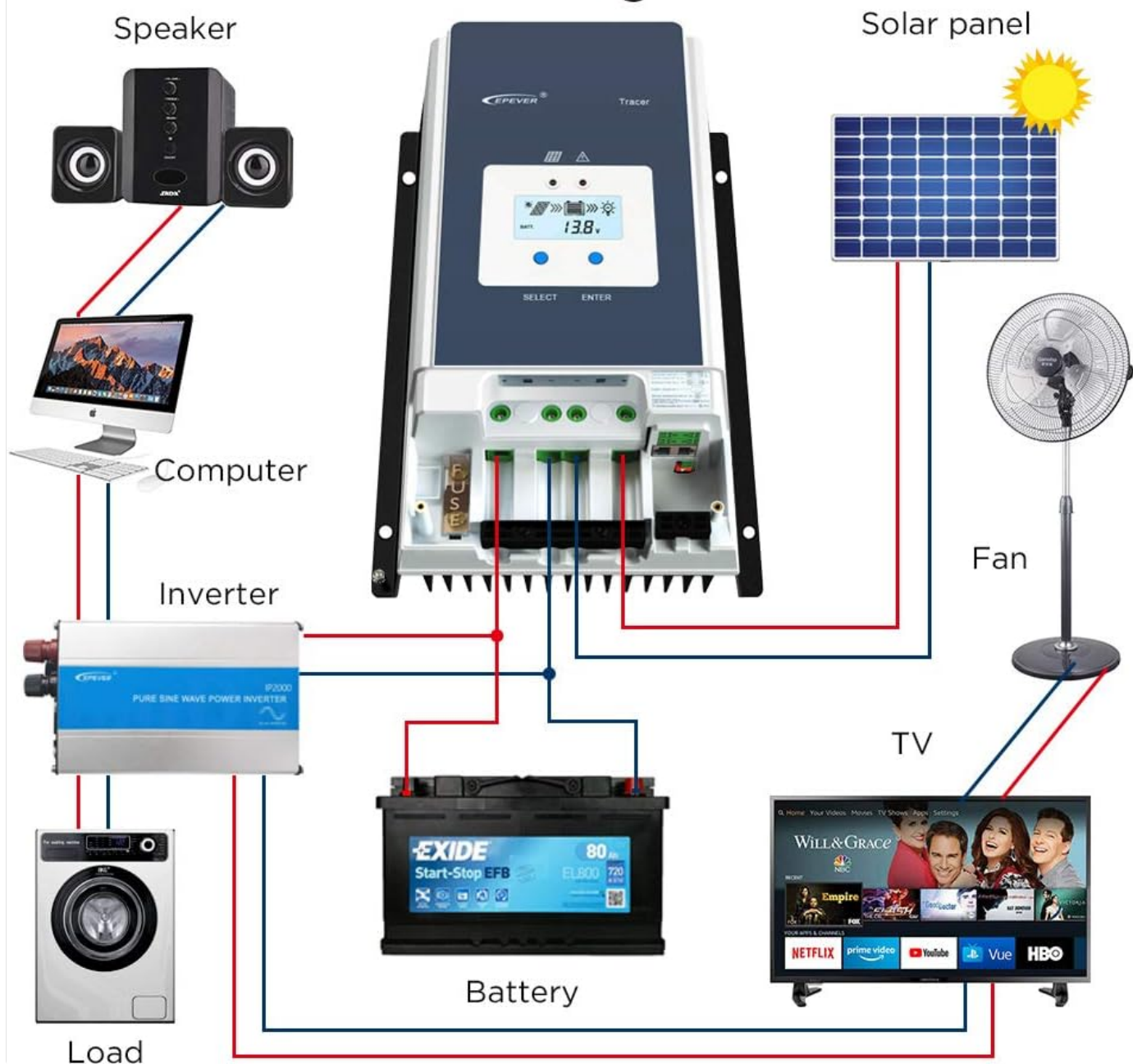
Image: Comprehensive wiring diagram showing the interconnection of solar panels, the EPEVER controller, battery, inverter, and various household appliances.
