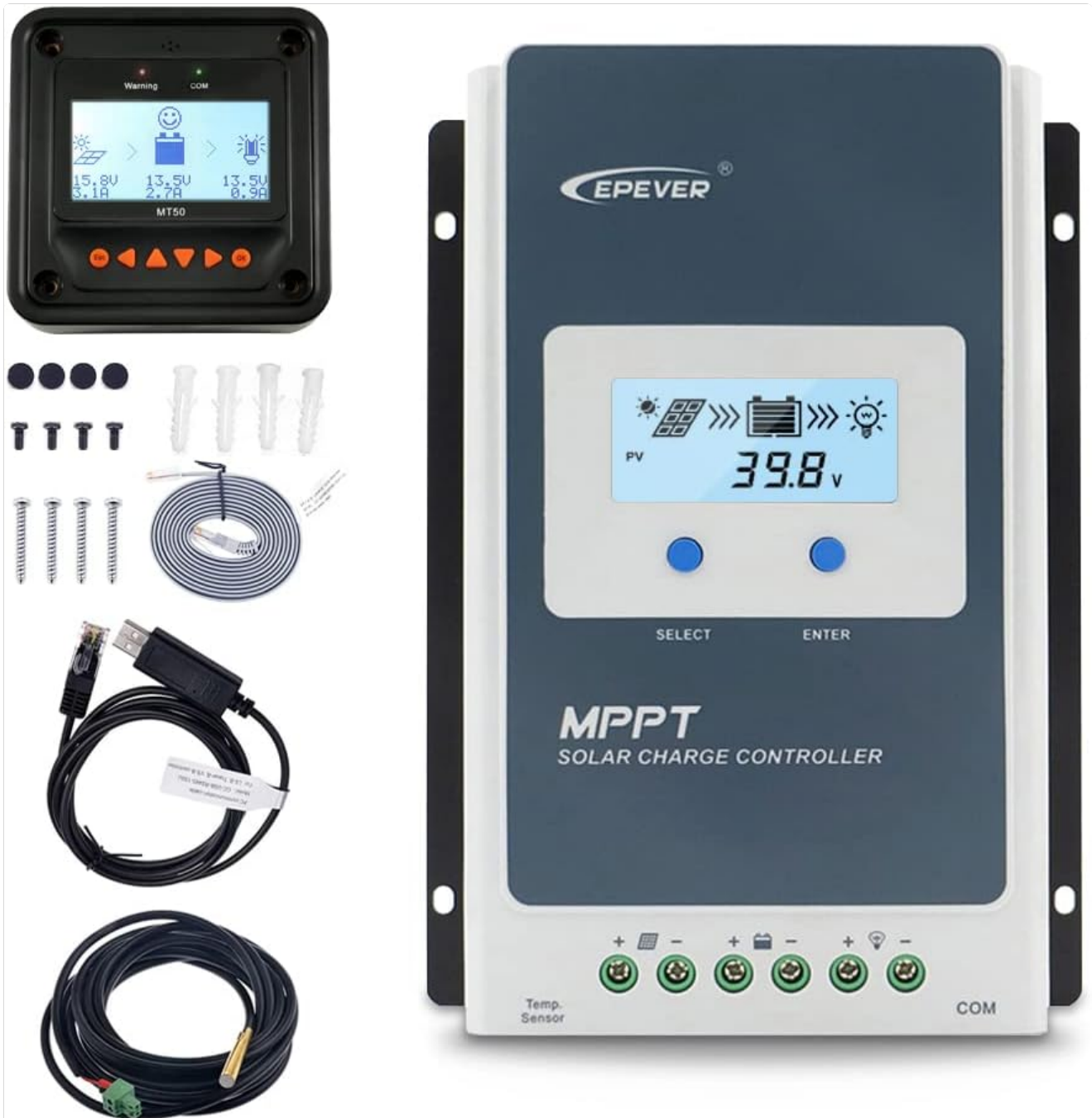
Figure 1: EPEVER Tracer3210AN Solar Charge Controller Kit Contents. This image displays the main controller unit, the MT50 remote meter, the remote temperature sensor, the PC communication cable, and mounting hardware.
