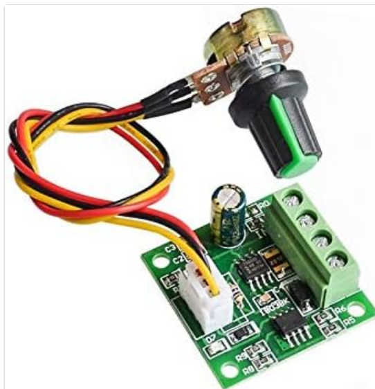
Figure 6.3: Example of the controller module connected to an external potentiometer for speed adjustment. The
