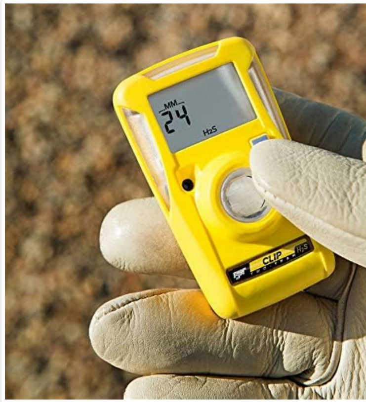
A hand wearing a work glove holding the yellow BW Technologies BW Clip H2S Monitor, displaying '24 MM H2S'.
