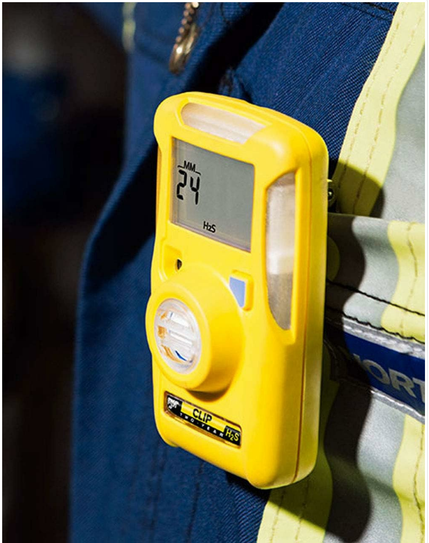
The yellow BW Technologies BW Clip H2S Monitor clipped onto a work uniform, showing its compact size and secure attachment.
