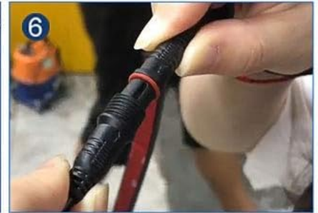
6. Connect the strips to the controller (arrow to arrow).
