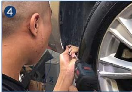
4. Open the inner fender and hide the extension cable.
