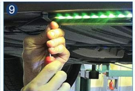
9. Test result. Use the buckles and screws to strengthen the firmness. Complete the installation.
