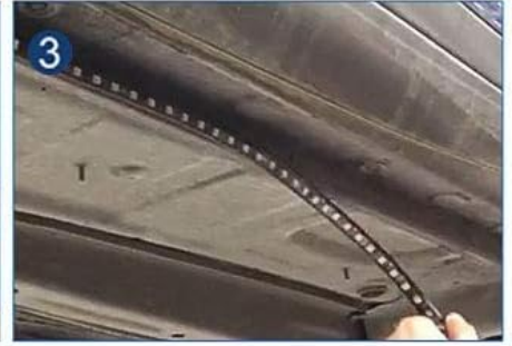
3. Peel off the 3M tape cover and stick it to the car .
