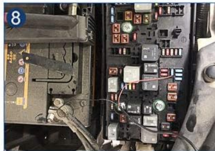
8. Connect the controller's power cord to the position of fog light. Red wire-Positive, black wire-Negative.
