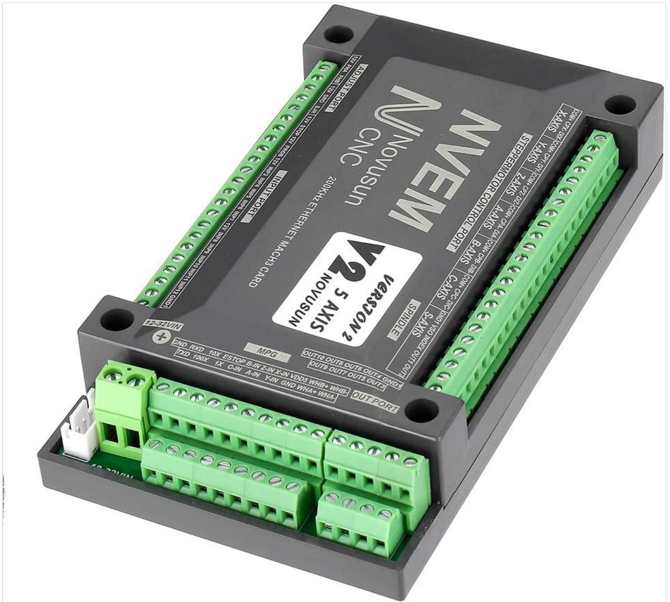
Figure 4.1: Angled view of the NVEM board, showing the 12-32V power input terminal and adjacent output terminals.
