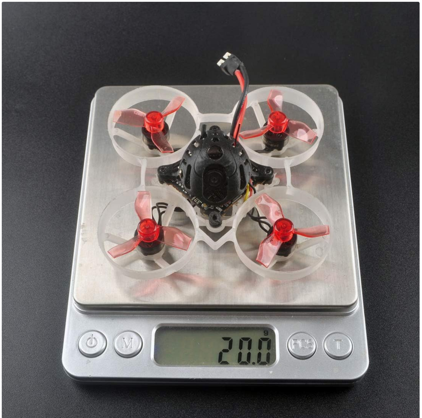
Figure 4: The Mobula6 drone on a digital scale, indicating a weight of 20.0 grams.
