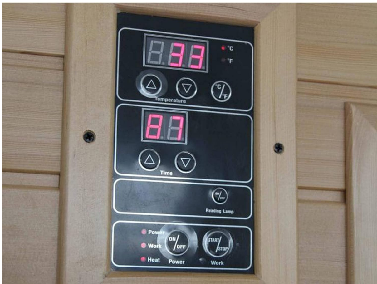
Figure 5: The external control panel features digital displays for temperature and time, along with buttons for adjustment, power, and reading lamp control.
