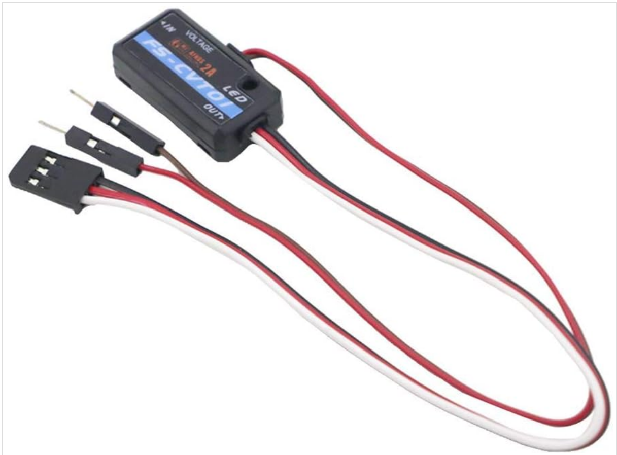
Figure 1: The Flysky FS-CVT01 voltage collection module with its input and output wires. The 3-pin connector plugs into the receiver, and the two bare wires connect to the voltage source.
