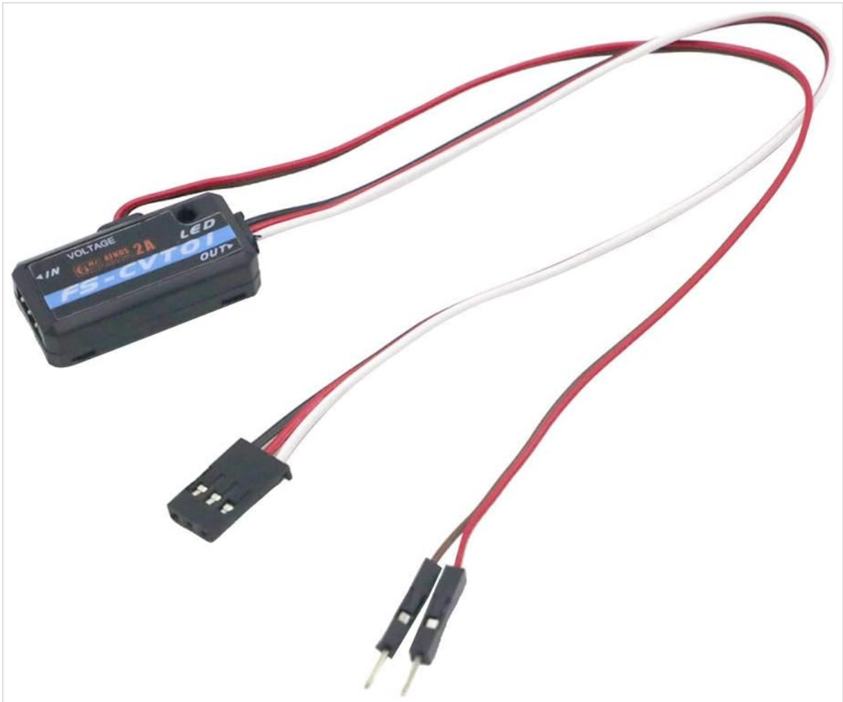
Figure 4: Top-down view of the FS-CVT01 module, showing its compact size and the clear labeling of its connections.
