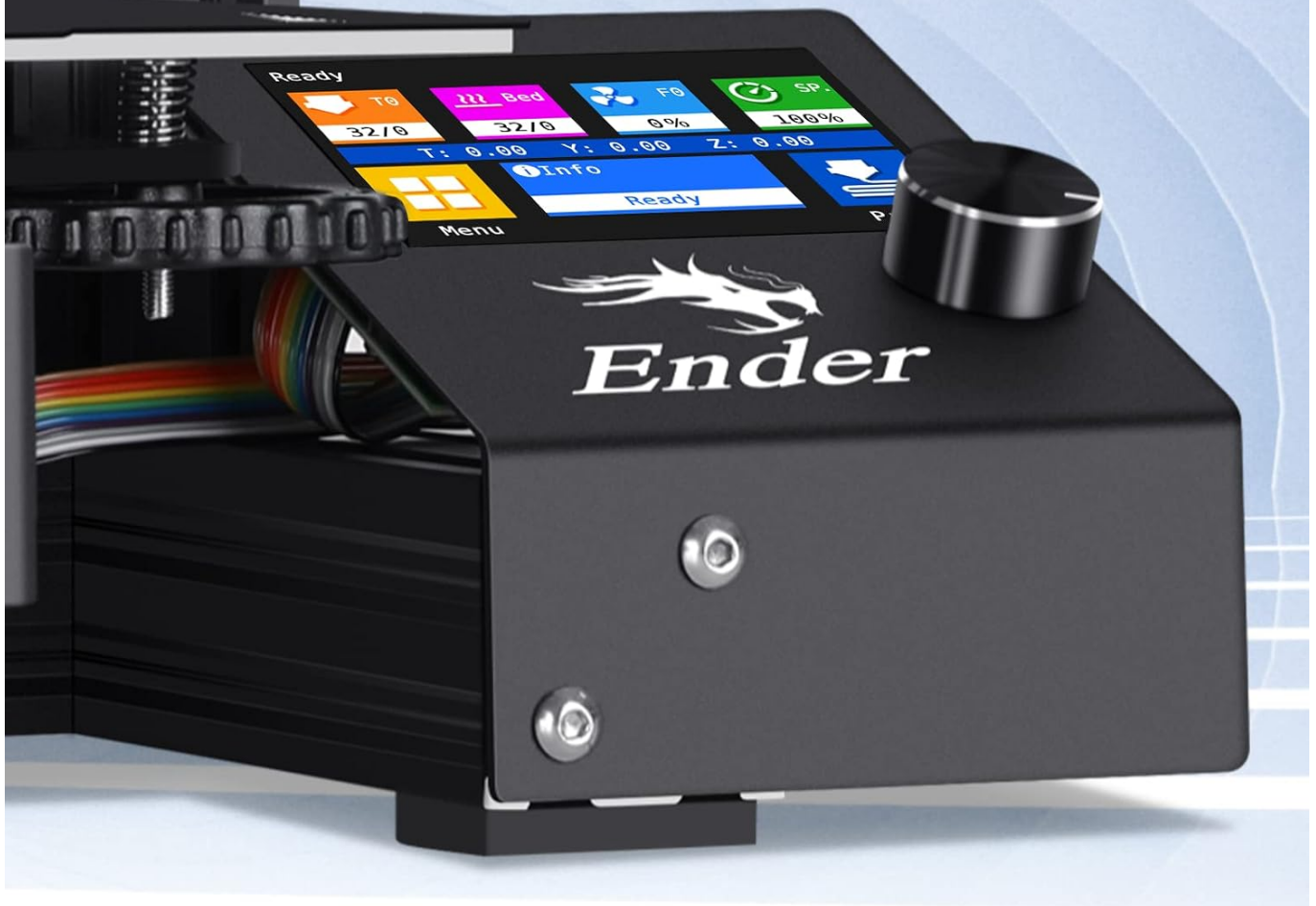
Image: Installation of the TFT35 E3 V3.0.1 display on an Ender 3 printer.
