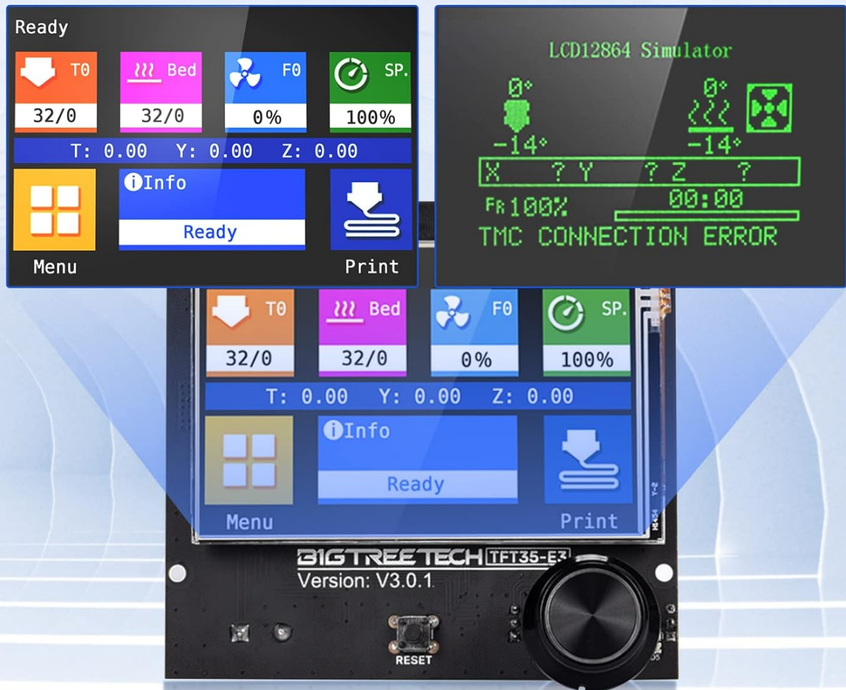
Image: The TFT35 E3 V3.0.1 display supporting both Touch and 12864 modes.
