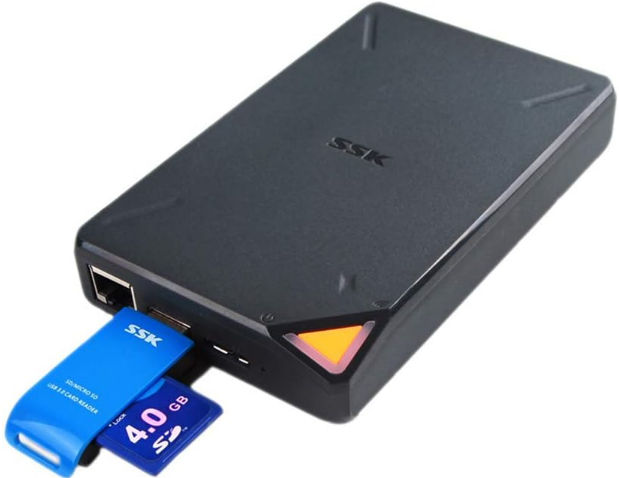
Image 4: The SSK SSM-F200 demonstrating its capacity expansion feature with an SD card reader and an SD card inserted into the USB Host port.
