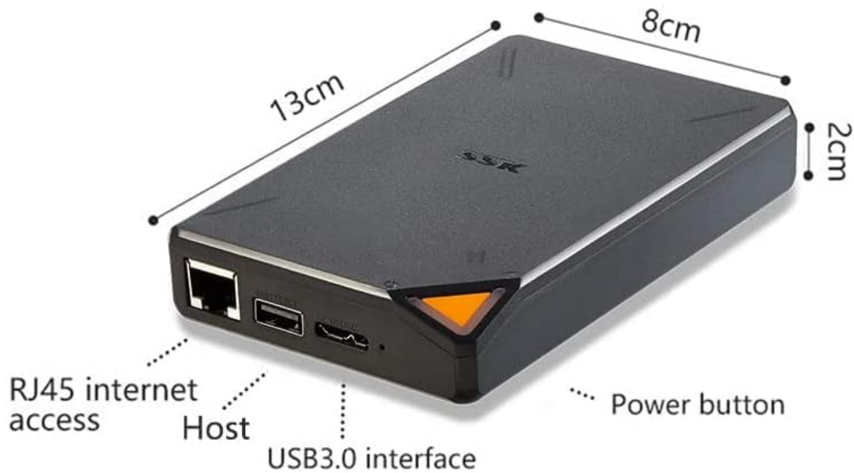
Image 1: The SSK SSM-F200 device showing its dimensions (13cm x 8cm x 2cm) and labeled ports including RJ45 internet access, USB Host, USB 3.0 interface, and the Power button.
