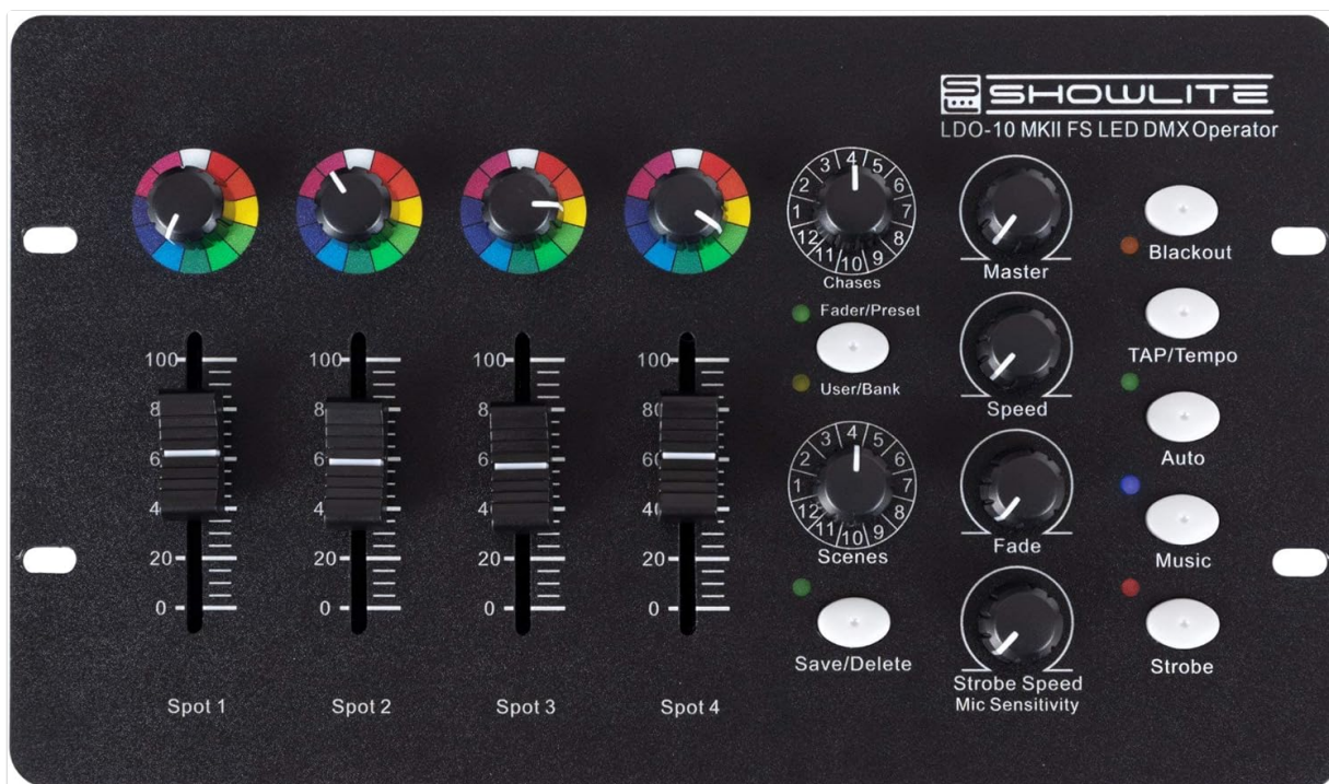
Image: The Showlite LDO-10 DMX MKII FS controller, featuring faders, rotary knobs for color and effects, and control buttons.
