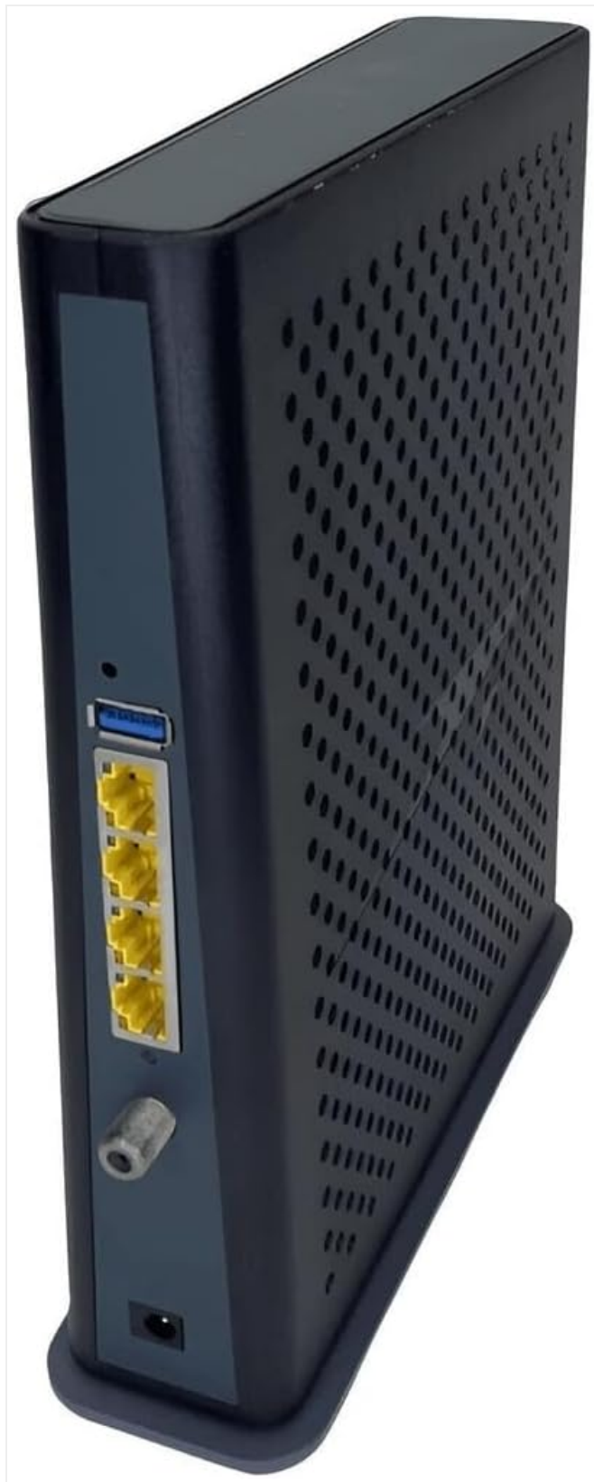
Image: Rear view of the Arris Touchstone DG3450, highlighting the coaxial cable input, four Gigabit Ethernet LAN ports, and the power input. A USB 3.0 port is also visible.
