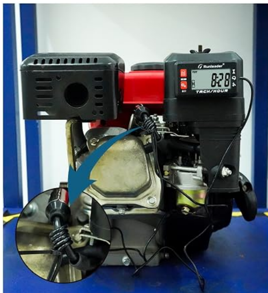
Image 3.2: Visual representation of both stick-on and screw-on mounting methods for the device.
