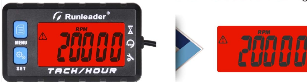
Image 4.3: Displays showing the maximum recorded RPM and the programmable RPM alert.
