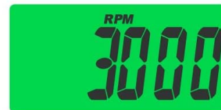
Image 4.1: The display showing total hours (TOT) when the engine is off, and real-time RPM when the engine is running.
