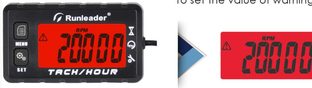
Figure 6: Top shows the "MAX RPM" recorded. Bottom shows the "ALERT RPM" setting, with a red backlight indicating a warning.
