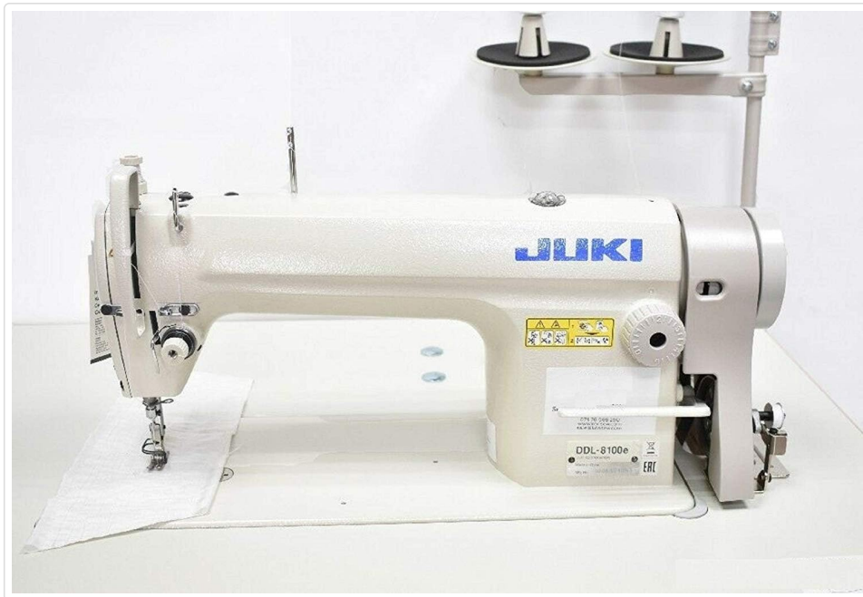
Figure 3.1: The JUKI DDL-8100 machine head, ready for operation.
