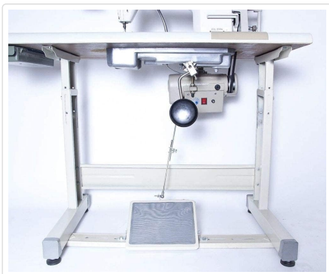
Figure 2.3: Underside view showing the motor and pedal connections to the machine.
