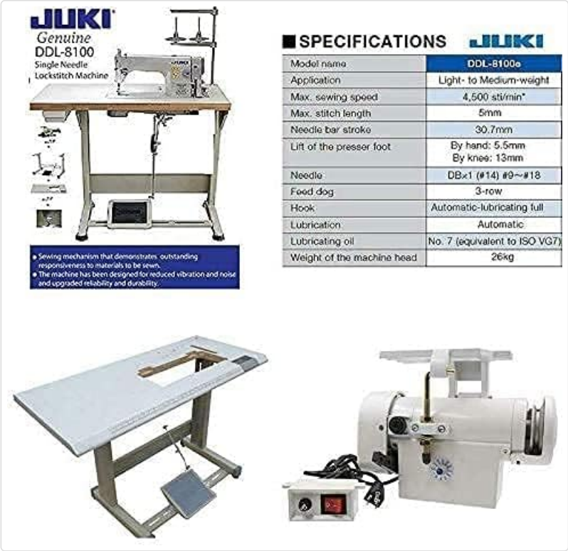
Figure 6.1: Official specifications diagram for the JUKI DDL-8100.
