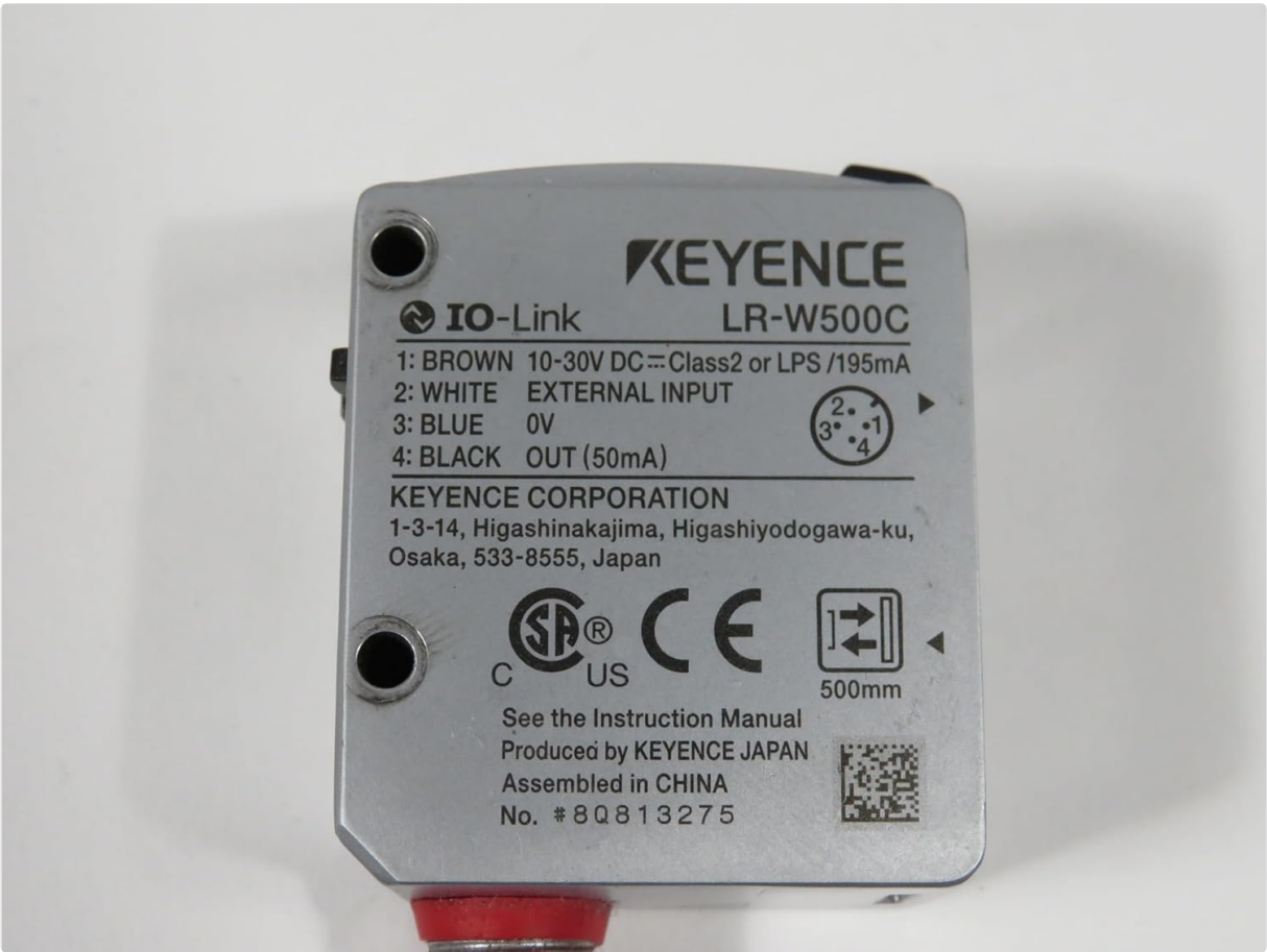
Figure 3.3: Back view of the Keyence LR-W500C sensor, displaying the wiring diagram for the 4-pin M12 connector and key product specifications.
