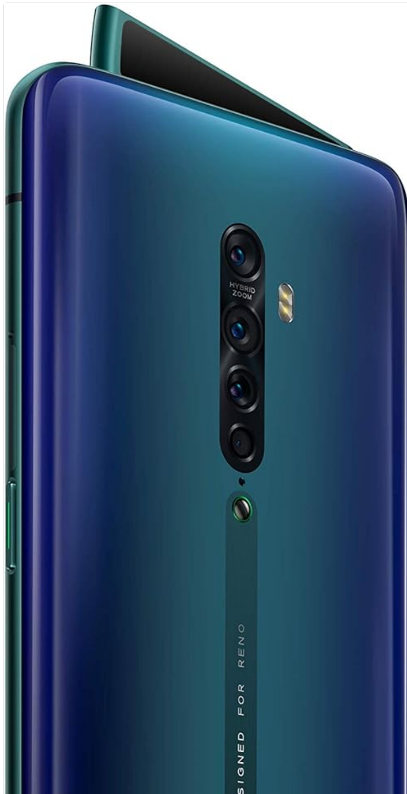
Figure 3.2: Side profile of the OPPO Reno2 CPH1907, highlighting the slim design and the mechanism of the pop-up front camera.
