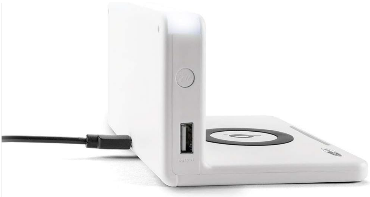
Image: Side view of the alarm clock, illustrating the power input port (left) and the USB output port (right).
