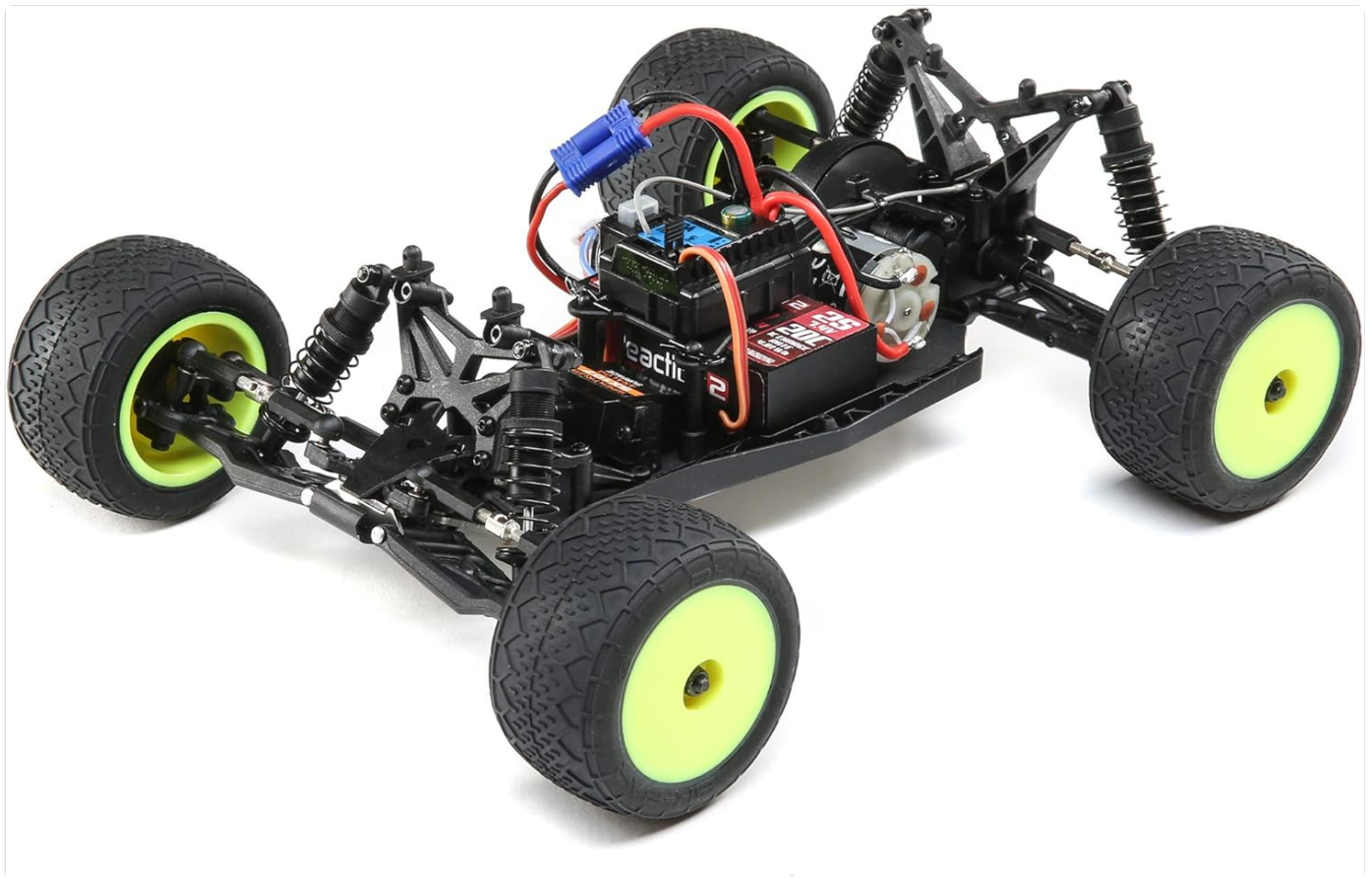
Image: The chassis of the Mini-T 2.0, illustrating the layout of the battery and electronic components.
