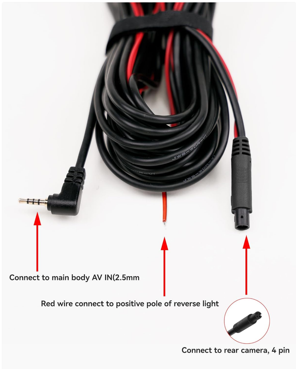
Figure 3.3: Connection points for the extension cable.
