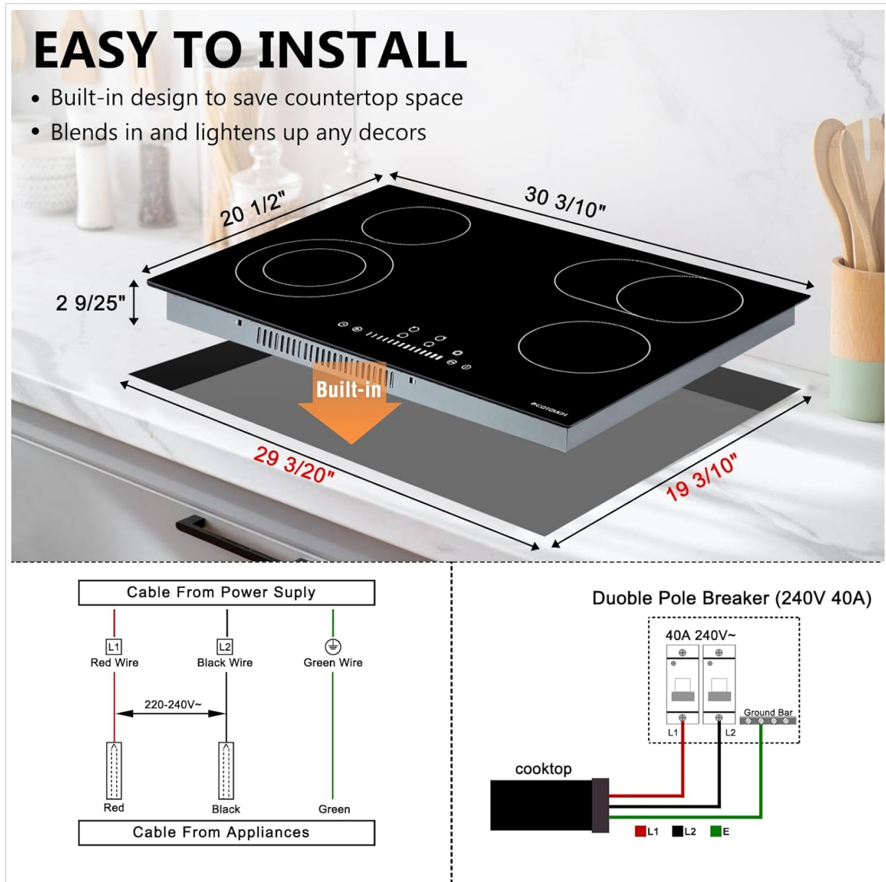
Image: Detailed installation diagram including product dimensions and electrical wiring instructions.
