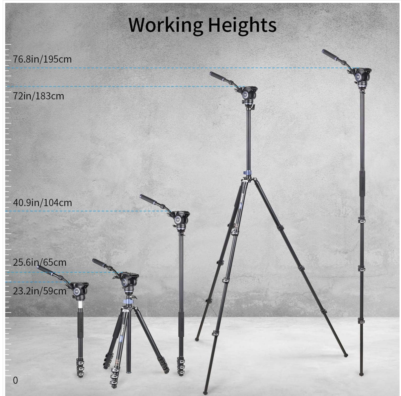
Figure 4.1: Illustrates the various working heights of the tripod, ranging from 59cm (23.2in) to 195cm (76.8in) with the center column fully extended.
