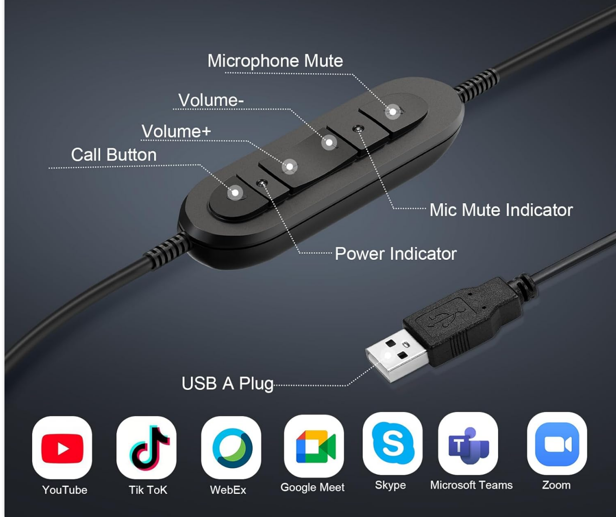
Image 4.1: Close-up view of the in-line control unit, highlighting the microphone mute, volume up/down, and call buttons, along with the mic mute and power indicators.
