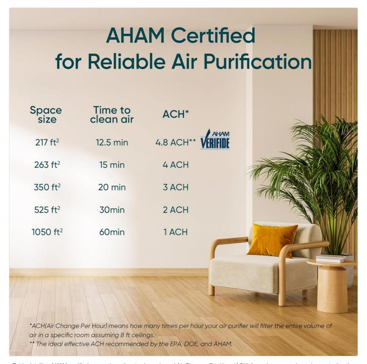
Table detailing AHAM certified space sizes, time to clean air, and Air Changes Per Hour (ACH) for various room sizes, demonstrating the purifier's efficiency.
