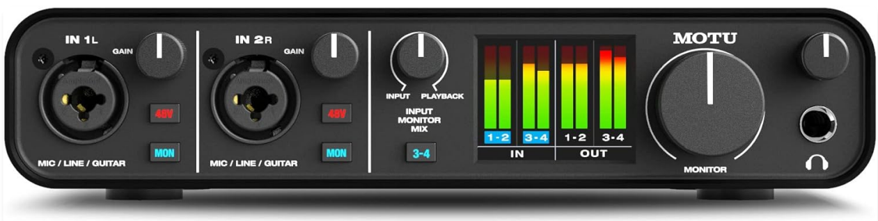
Image 3.1: Detailed view of the MOTU M4 front panel controls.
