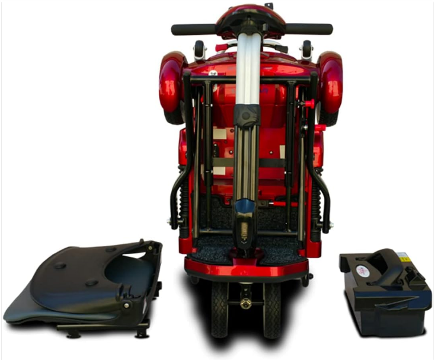
Figure 3: The EV Rider Transport Plus scooter in its fully folded configuration, alongside its removable seat and battery pack, demonstrating its portability.
