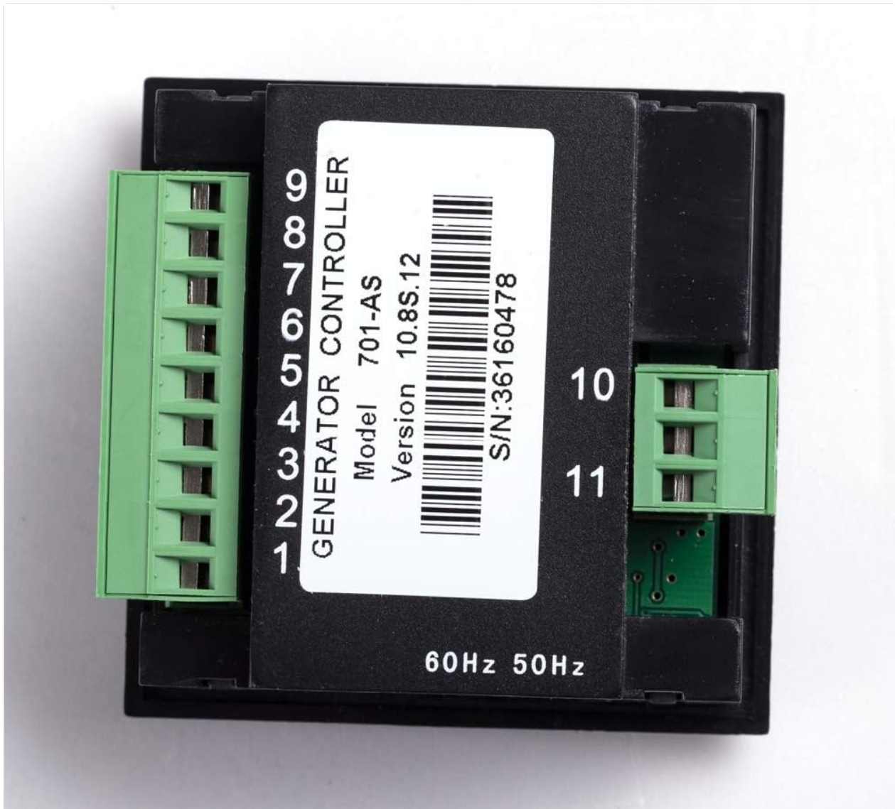
Figure 3.1: Rear view of the DSE701K-AS controller, displaying the terminal blocks for electrical connections. Numbers 1-9 are visible on the left block, and 10-11 on the right block, indicating connection points for various generator functions and sensors.
