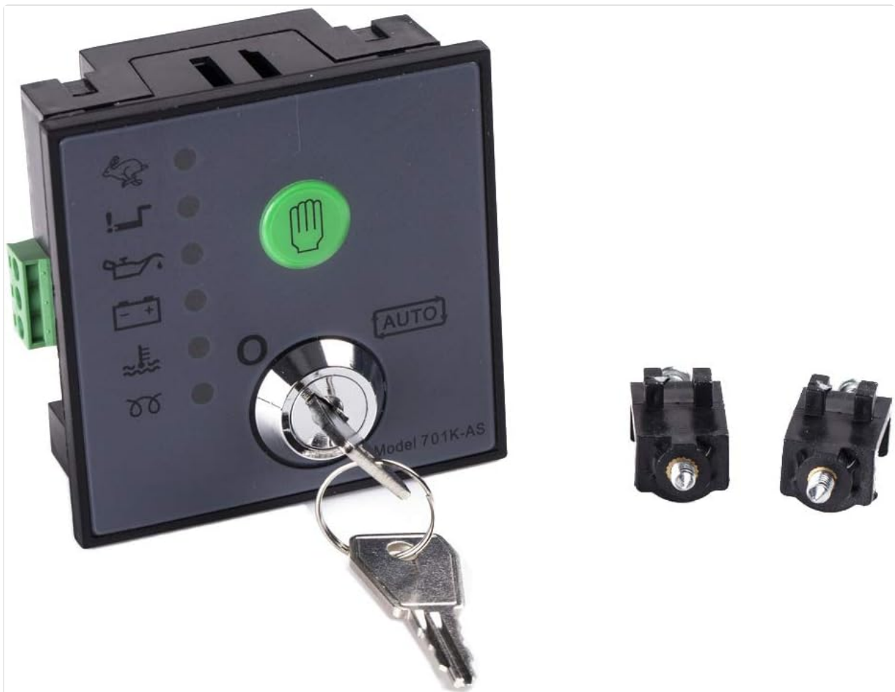
Figure 4.1: The DSE701K-AS controller shown with its accompanying keys. The front panel features a green AUTO button, a key switch, and a series of LED indicators for monitoring engine parameters such as oil pressure, battery, and temperature.
