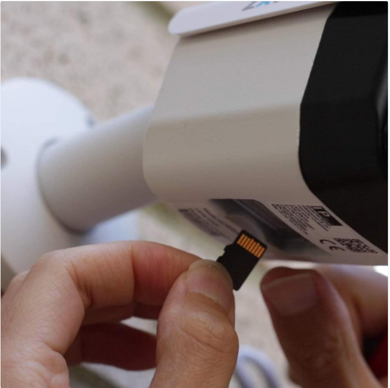
Image: A hand inserting a microSD card into the camera's external slot, demonstrating the process for local storage setup.
