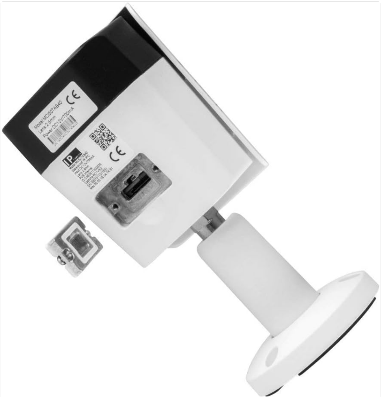
Image: Rear view of the camera, highlighting the external SD card slot and the robust mounting bracket.
