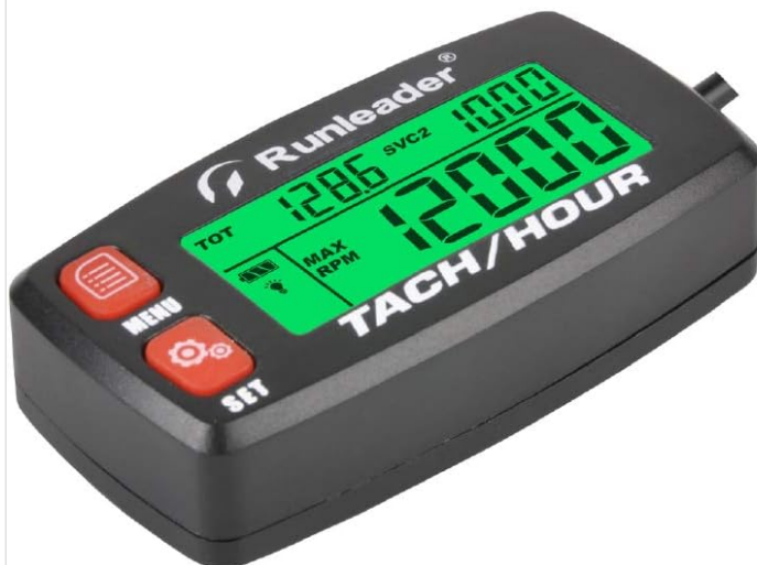
Figure 3: Display illustrating SVC and SVC2 countdown tracking for maintenance reminders.
