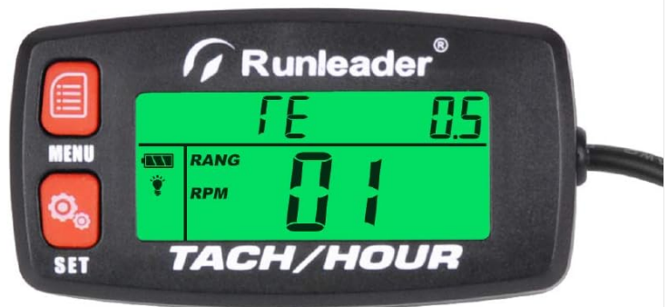
Figure 10: Display showing programmable firing patterns for different engine types.
