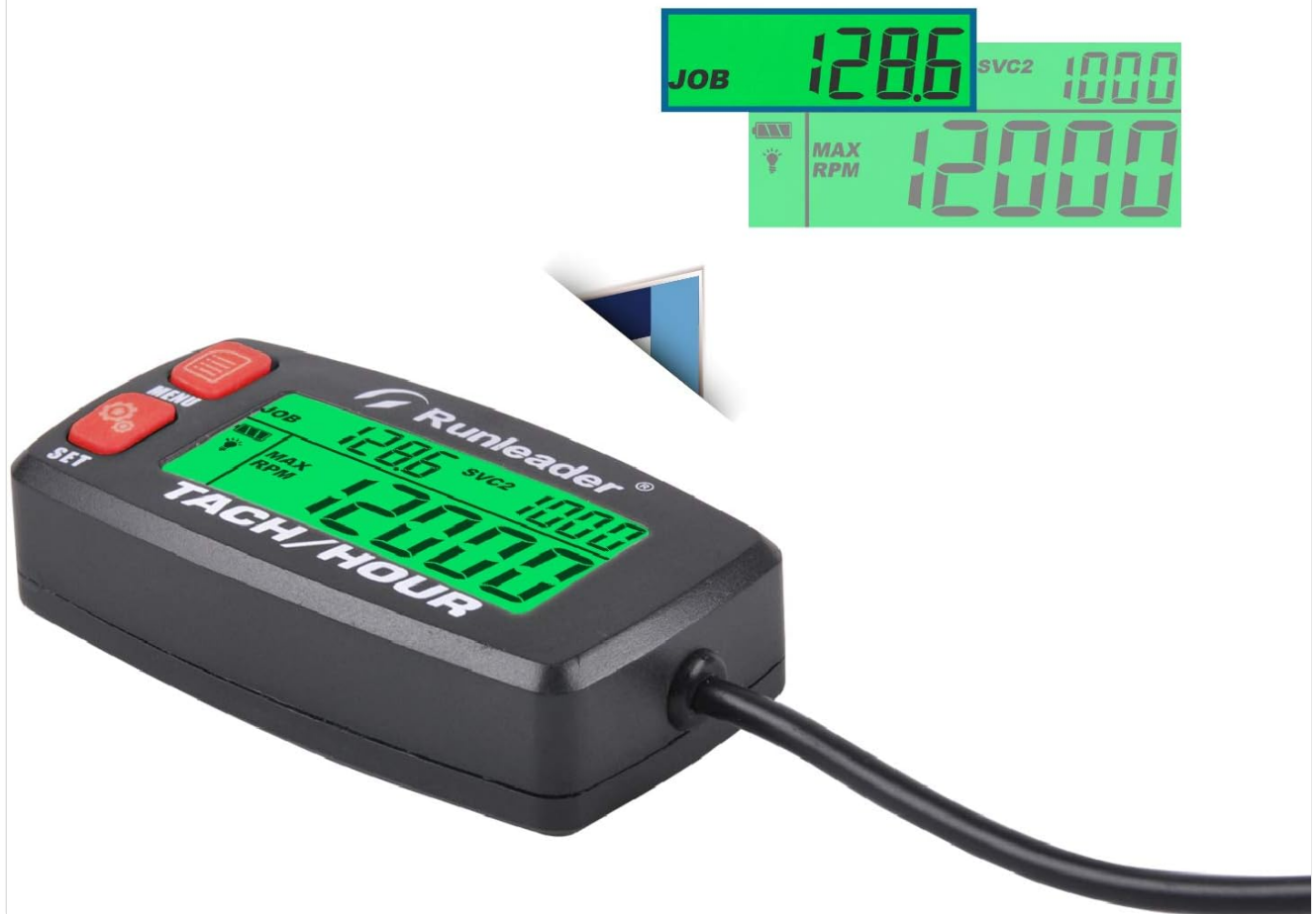
Figure 4: Display showing the Job Timer function for measuring specific work durations.
