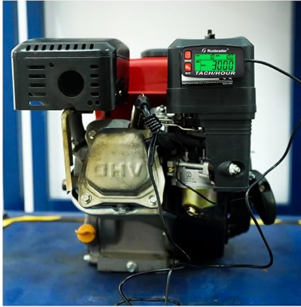
Figure 8: Illustration of engine signal wire connection and available mounting methods.
