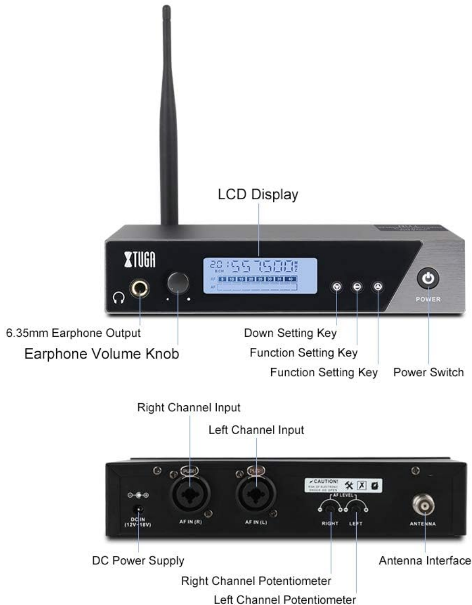
Image 4.1: Detailed diagram of the XTUGA IEM1100 Wireless Transmitter, showing the front panel with LCD display, earphone output, volume knob, setting keys, and power switch. The rear panel illustrates the DC power supply input, AF inputs (Left/Right), and antenna interface.
