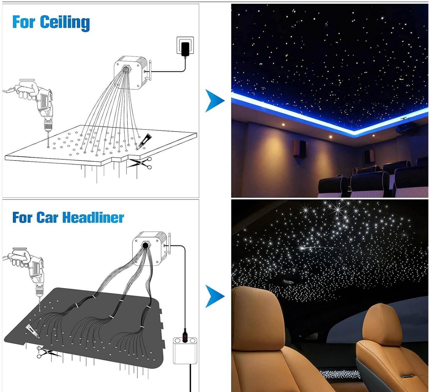
Image 5.1: Installation diagram for both ceiling and car headliner applications.
