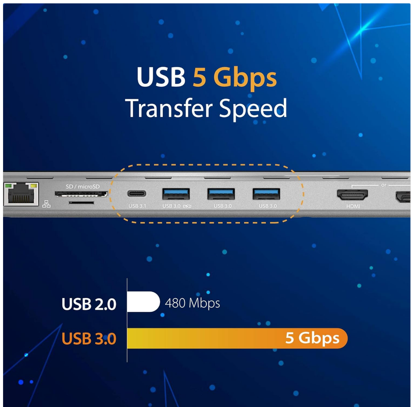
Figure 4.5: Comparison of USB 3.0 (5 Gbps) and USB 2.0 (480 Mbps) transfer speeds.
