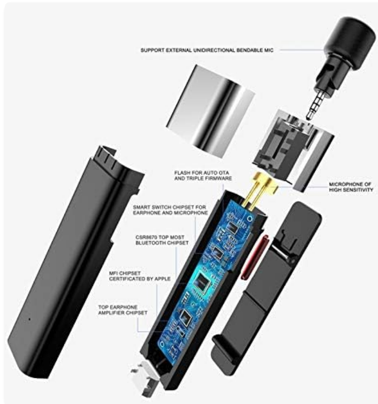
Figure 3: Exploded view of the SmartMike+ revealing its internal components. Key parts highlighted include the high-sensitivity microphone, CSR8670 Bluetooth chipset, MFI certified chipset, and top earphone amplifier chipset.
