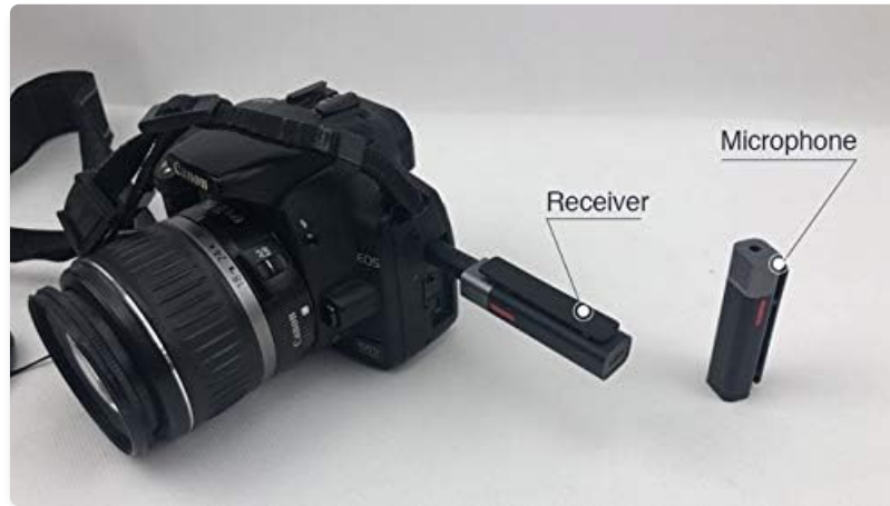
Figure 4: The SmartMike+ acting as a receiver connected to a DSLR camera, with a second SmartMike+ unit shown as the microphone. This illustrates a typical setup for recording audio directly to a camera.
