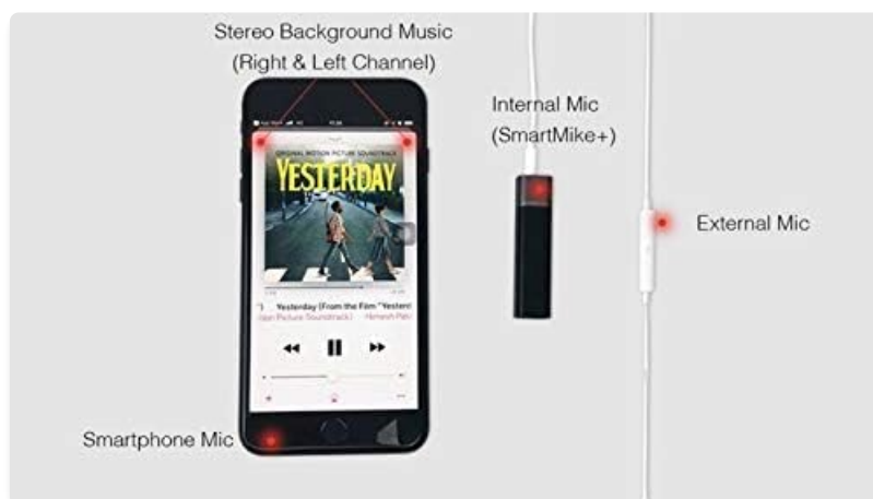
Figure 5: Diagram illustrating audio input options with the SmartMike+. It shows how stereo background music, the internal SmartMike+ microphone, an external microphone, and the smartphone's built-in microphone can all contribute to the audio input.
