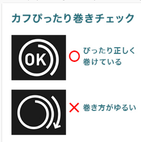
Image: Visual representation of the 'Cuff Fit Check' feature, showing the 'OK' symbol for a correct fit and a warning symbol for a loose fit.
