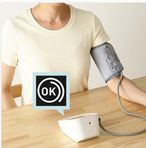
Image: The blood pressure monitor display showing an 'OK' symbol, indicating the cuff is correctly wrapped.
