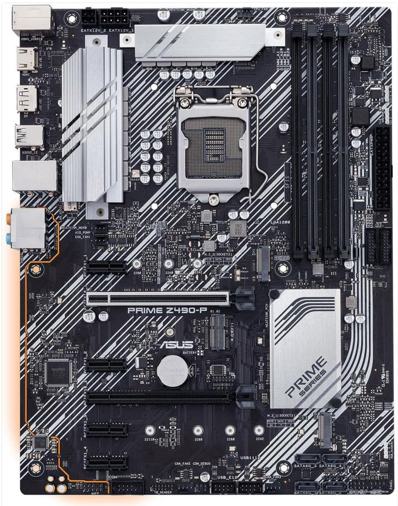
Image: Top-down view of the ASUS Prime Z490-P motherboard, highlighting key component locations such as the CPU socket, DIMM slots, PCIe slots, and M.2 slots.
