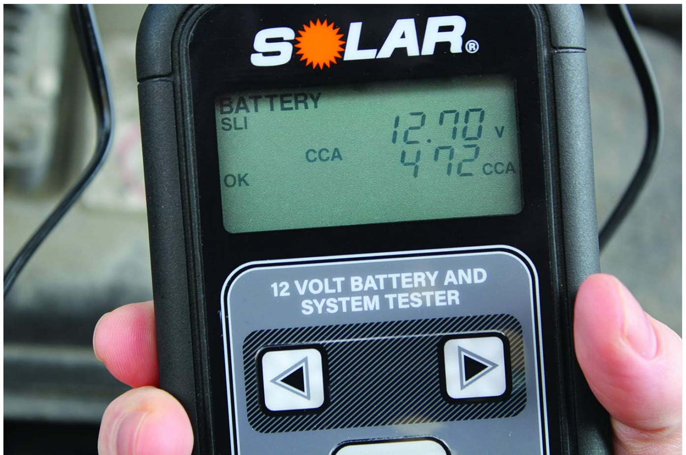
Figure 3: The BA6 display showing battery type (SLI), CCA, voltage, and an "OK" status.
