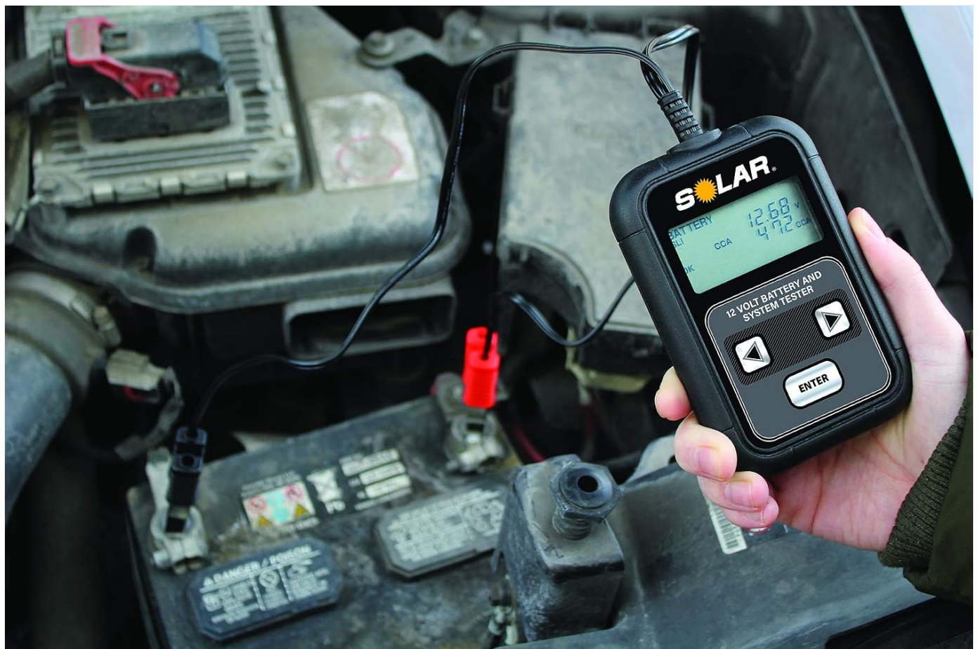
Figure 2: The BA6 tester connected to a vehicle battery for testing.
