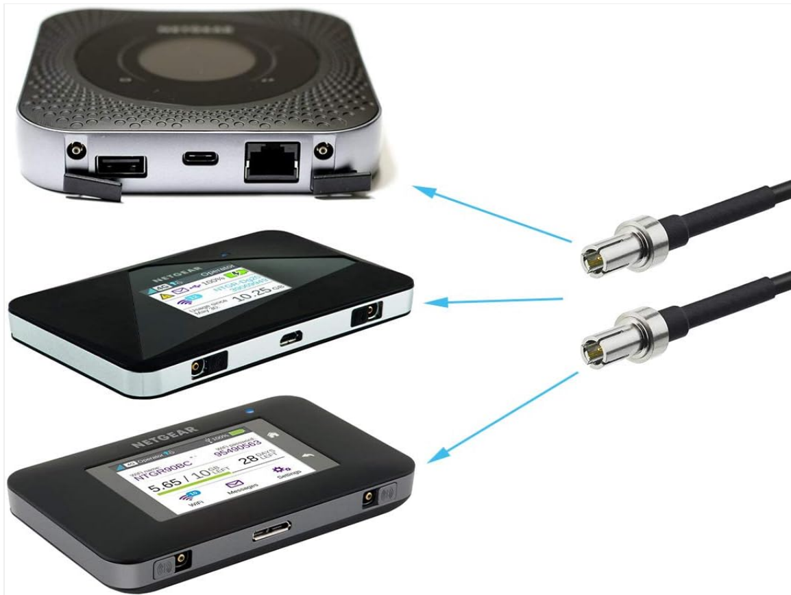
Image 4.2: Connection of antennas to compatible devices. This image illustrates how the antennas connect to different models of mobile hotspots and routers.
