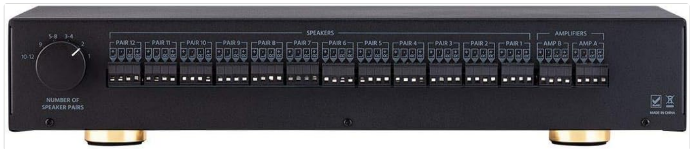
Figure 4.2: Rear panel of the Monoprice SS-Pro 12. Shows input terminals for two amplifiers (AMP A, AMP B), output terminals for twelve speaker pairs (PAIR 1-12), and a rotary switch for "NUMBER OF SPEAKER PAIRS" with settings 3-4, 5-8, 9-12.
