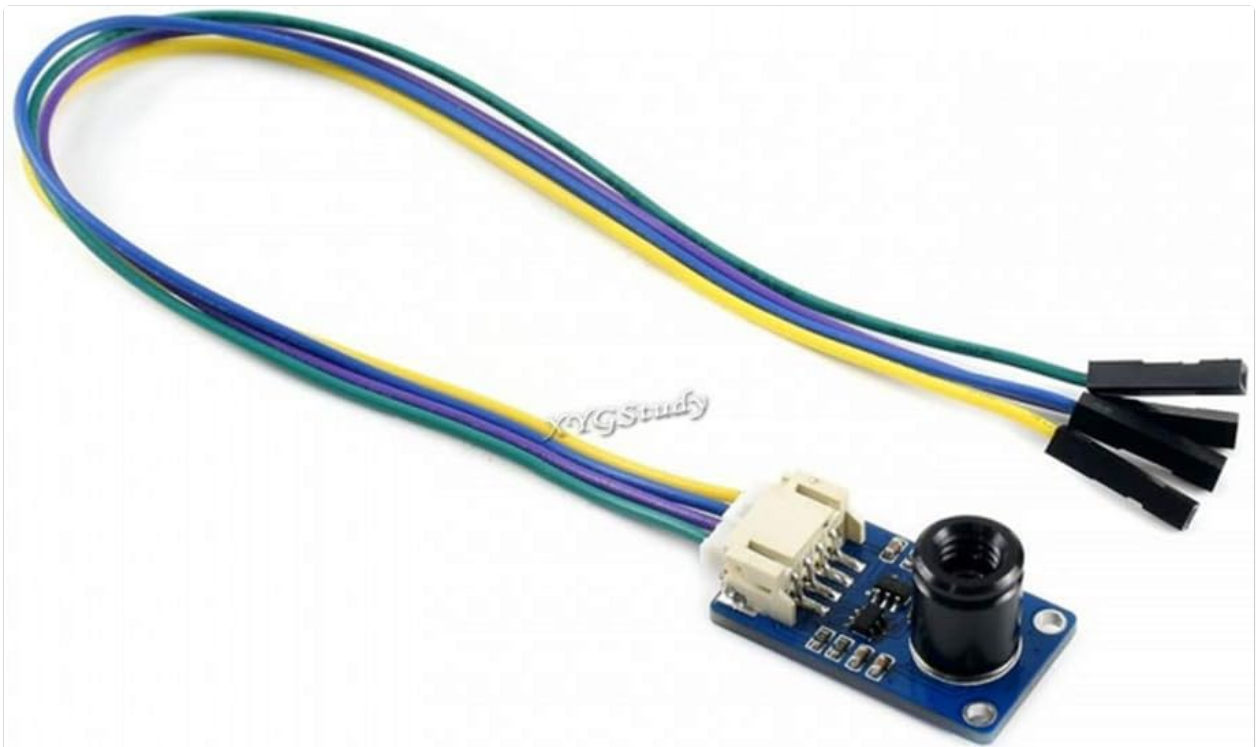
Figure 5: The MLX90640-D55 module connected with its 4-pin wire.
