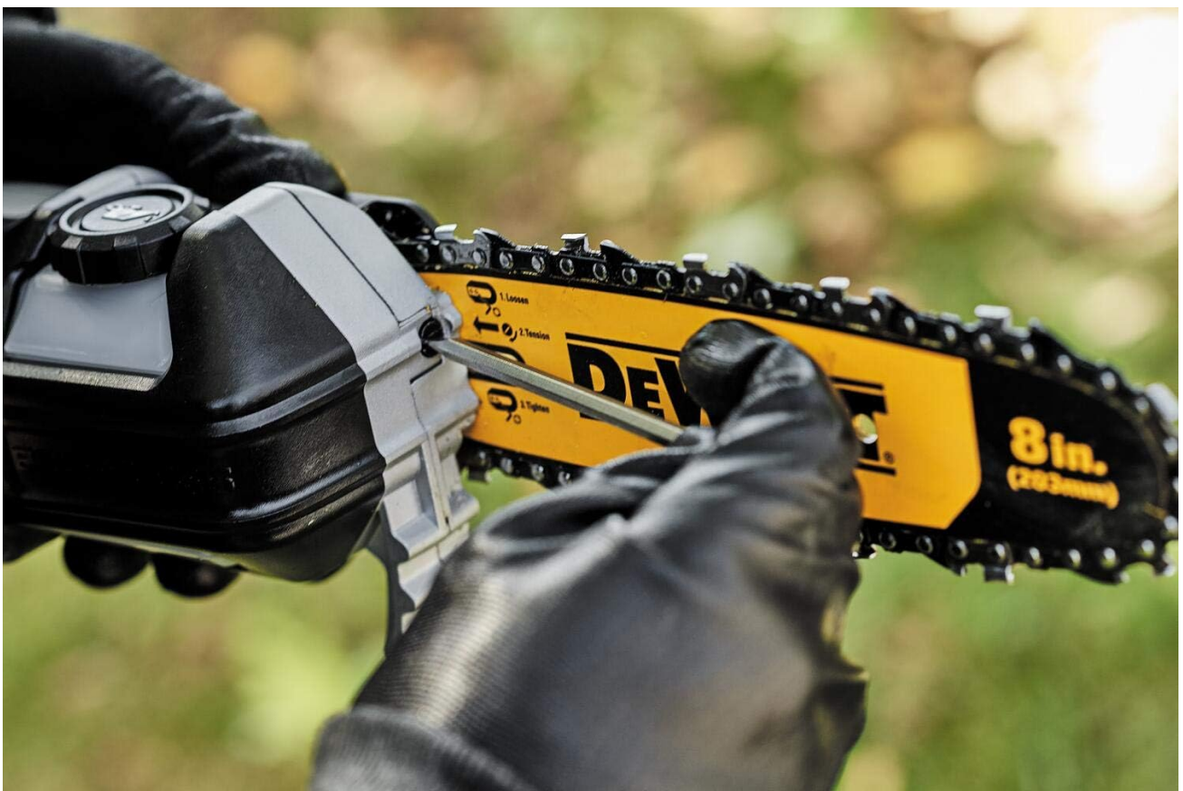
Figure 3.4.1: A close-up view of a hand using a hex wrench to adjust the chain tension on the pole saw's cutting head.
