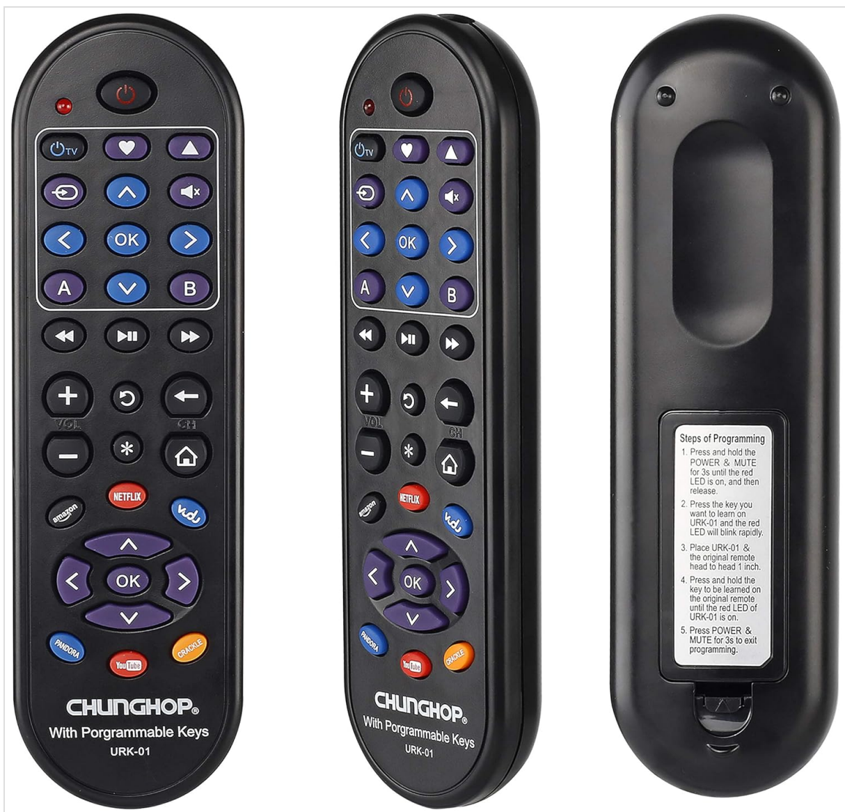
Image: Front, side, and back views of the CHUNGHOP URK-01 Universal Remote Control. The front shows various buttons including power, navigation, volume, channel, and dedicated streaming service buttons. The back shows the battery compartment cover.
