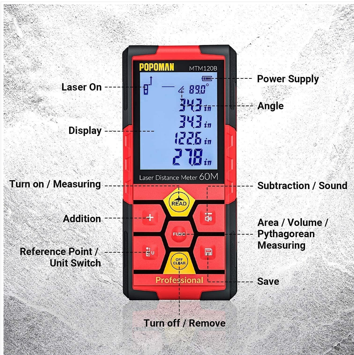
Figure 4.1: Front view of the POPOMAN MTM120B Laser Distance Meter with key components labeled.
