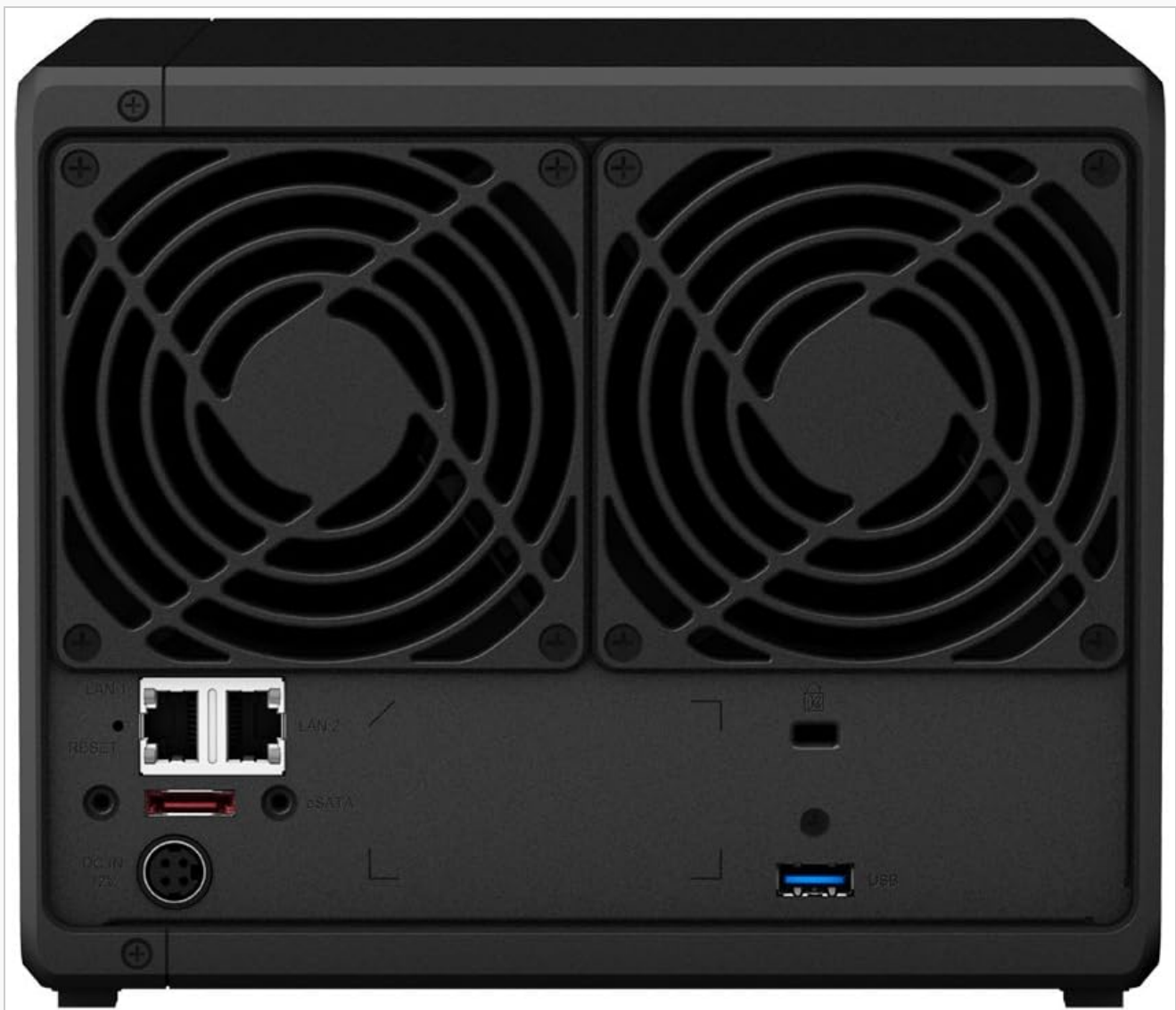
Figure 2: Synology DiskStation DS918+ Rear View. This image highlights the rear panel, displaying two RJ-45 1GbE LAN ports, two USB 3.0 ports, one eSATA port, the power input, and dual cooling fans.
