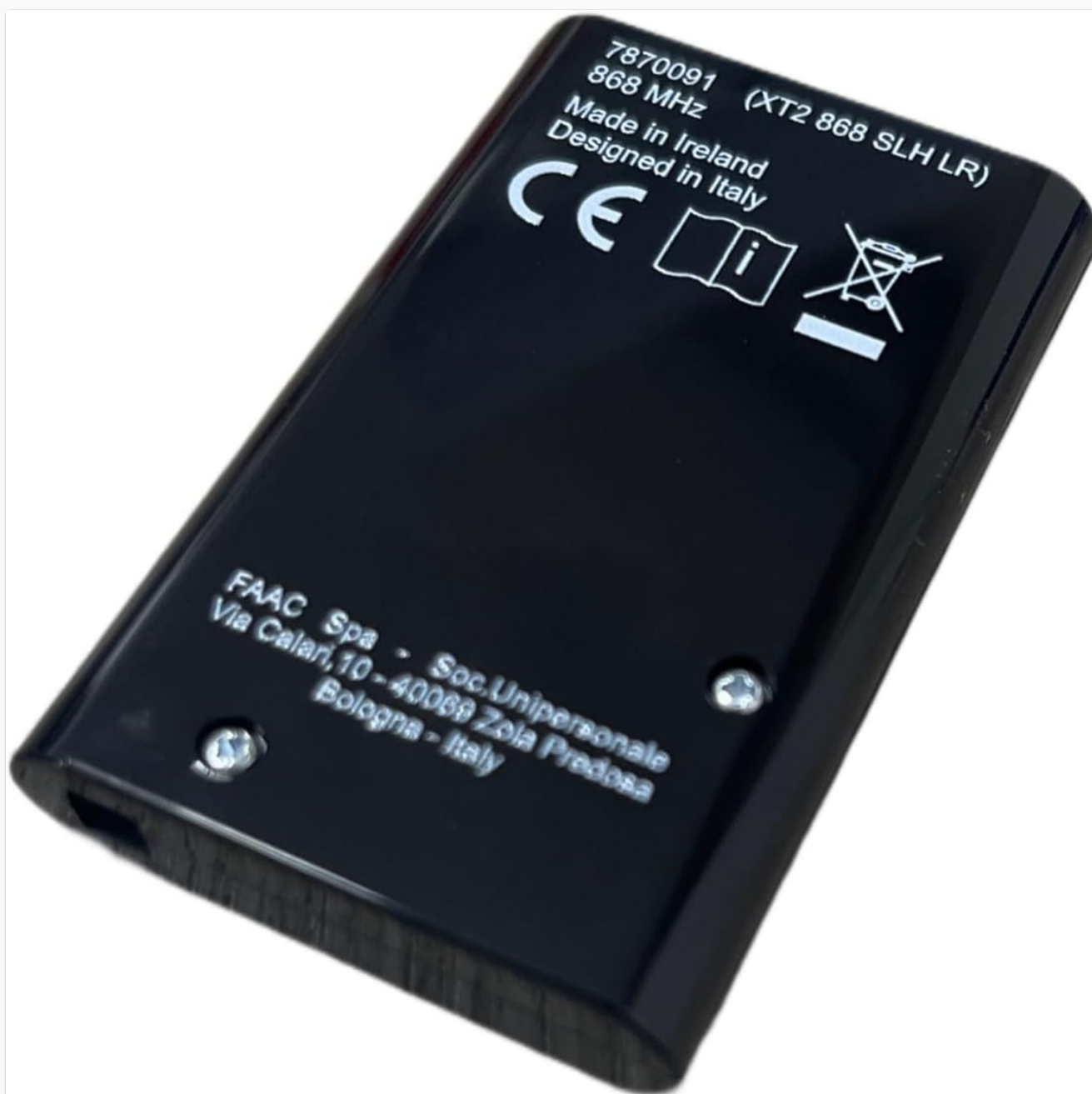
Image 5.1: Back view of the remote control, showing the location of the screws for accessing the internal components, including the battery. The product label with model and frequency information is also visible.
