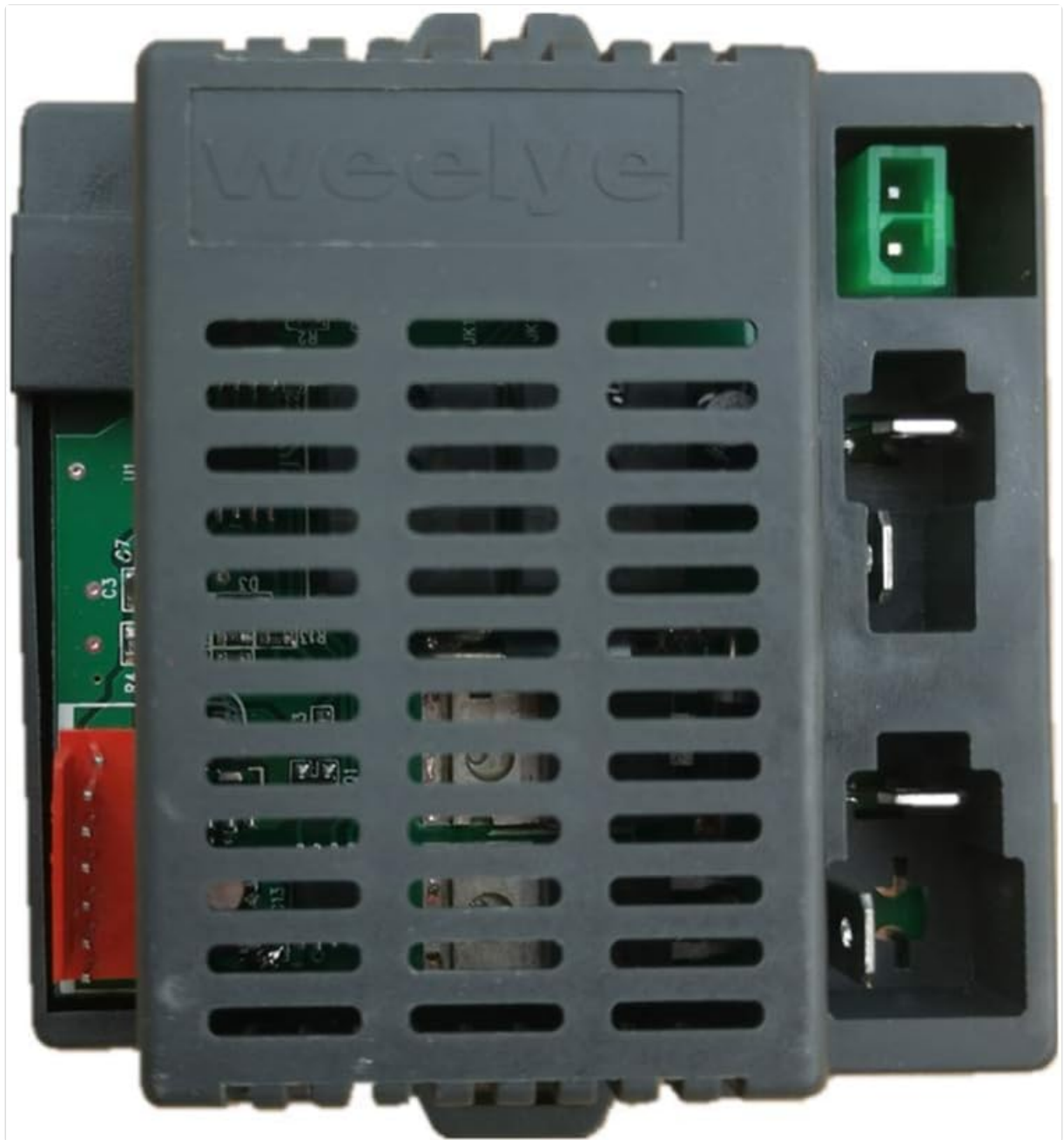
Image: Close-up of the weelye control box, showing its design and connection ports. This view helps in verifying the physical match with your existing unit.
