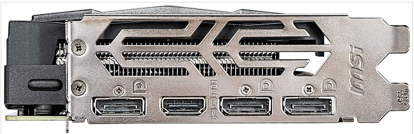
Image 4.2: Rear view of the graphics card, displaying the DisplayPort and HDMI output connectors.
