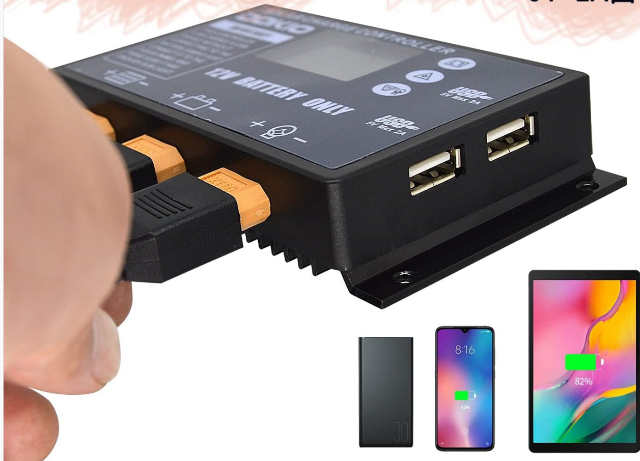
Figure 2: The controller features dual USB ports for charging various devices.
